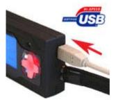
The R-300/500 Wideband Computer contains an onboard USB port. Although interface is made via USB port, from the perspective of the software developer, this port can be treated as a standard serial COM port. To find out which COM port the R-300/500 is assigned to, go to "Start" > "Control Panel" > "Systems" > "Hardware" > "Devices Manager" and look under the "Ports" tab.
